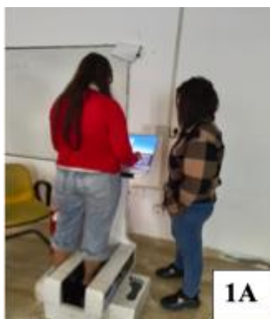
Figures 1 (a and b): Assessment of bilateral foot anthropometric dimensions using a 3D foot scanner (LSF-350-A): (a) participant positioning and (b) digital foot measurement output. scanner.
